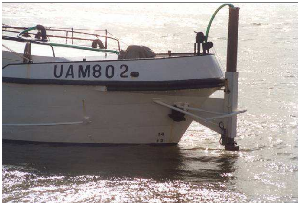
Fig. 3.19 "Transducer installation over the bow"
